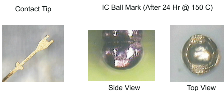
Figure 6-7. Micro Tuning Fork Contact and Contact Marks on Solder Balls
