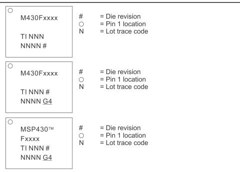
NOTE: Package marking with "TM" applies only to devices released after 2011.
