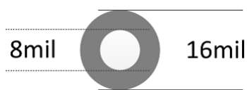
Figure 11-7. Recommended Minimum Via Sizing
